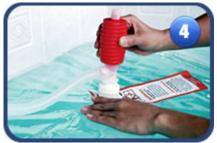
the center nozzle cap and thread on the siphon pump by turning in a clockwise motion.
