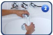
Unscrew the nozzle cap that is closest to the faucet and attach the fill sock to that nozzle by turning it clockwise until tight. Slide the other end of the fill sock over the bathtub faucet.
